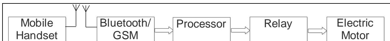
Fig 4: Block diagram of Bluetooth controlled electric motor
